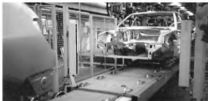
Picture left: Safety provisions for a production conveyor at an automobile manufacturer by means of a safety light barrier
